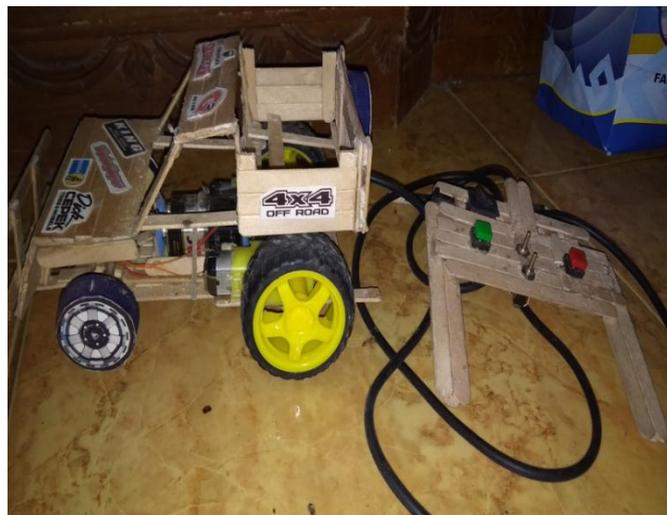
Gambar 4.6 Tampilan Mobil Remote Control Sederhana
