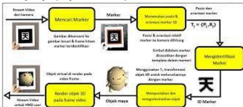
Gambar 2. 1 Prinsip Kerja Augmented Reality
